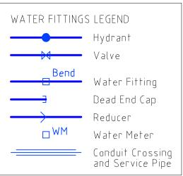
(1) Ø150 11.25° Bend (2) Ø150 22.5° Bend (3) Ø150 45° Bend (4) Ø150 90° Bend (5) Ø150 Dead End Cap 6 Ø150 Hydrant (7) Ø150 Valve (8) Ø150 x Ø150 Tee (9) Ø225 11.25° Bend
